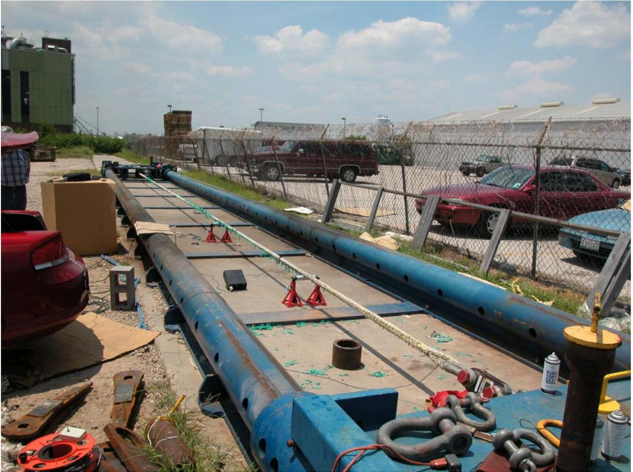
**A.4 Dillon load cell shackled between the hydraulic cylinder and the eye splice of the 38mm diameter tow rope.**
