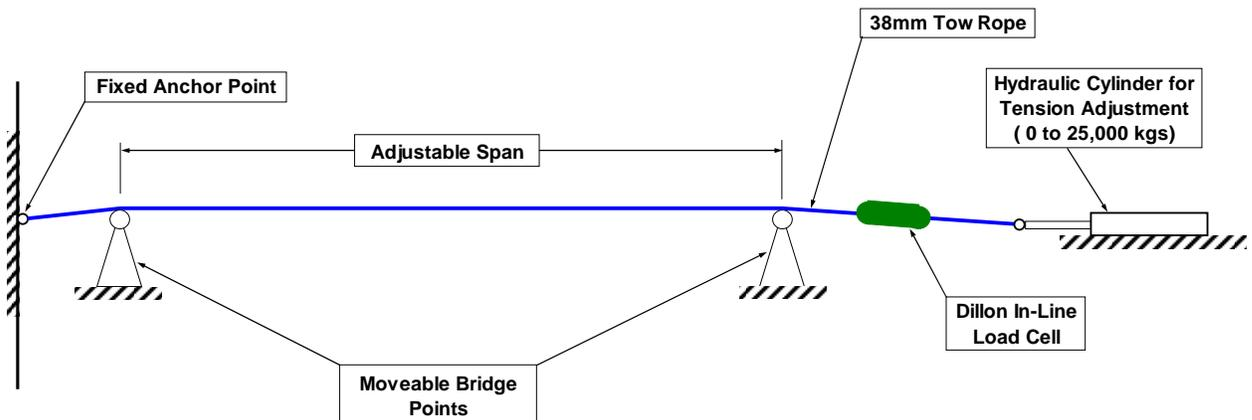
The Viten P1000 consists of a main electronics box, with a remote single axis accelerometer that gets affixed to the tow rope at any point between the two moveable bridge points. The tow rope is excited manually (using a gentle tap with a rubber mallet), allowing the accelerometer to sense the natural frequency of the vibration response of the rope under tension. From the natural frequency, tension can be inferred as follows:
